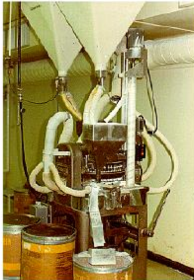
Figure 3.13 Tablet press with load hopper and spiral dust pickups for product recovery
